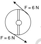
Assuming that the streering wheel has a diameter of 400 mm, determine the moment associated with these forces.
